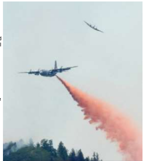
A lead plane, like the one flown by Col. Paul Delmonte, peels off after directing a MAFFS-equipped C-130 to a drop zone over a forest fire (U.S. Air Force photo)
