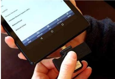
A RIO Connect user inserts a mobile CAC reader into an Android tablet in order to gain access to CAC-secured websites.
